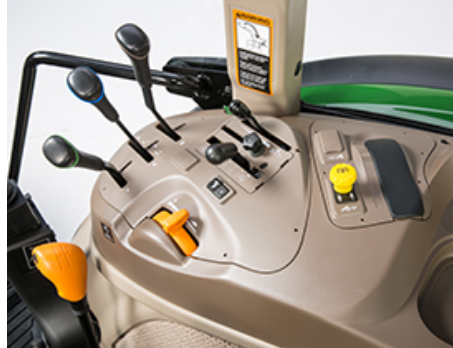
Hitch control levers - Cab
