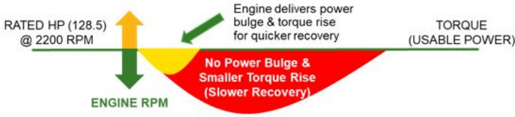
Power bulge and torque curve
