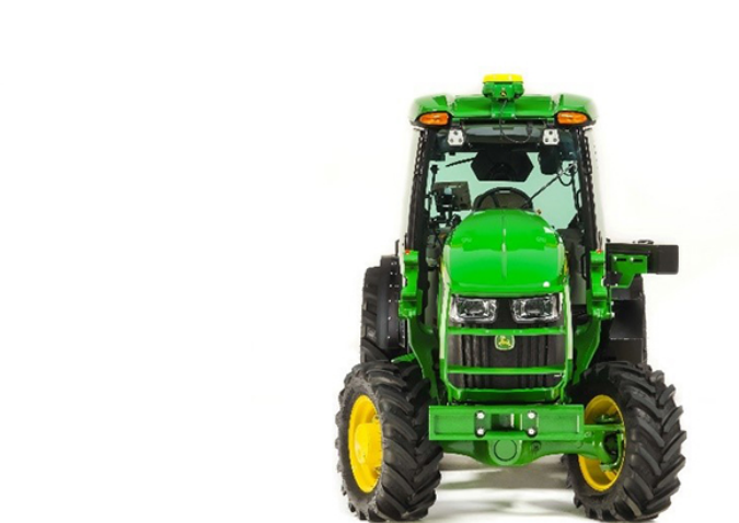
Narrow MFWD Axle on 5ML Cab
